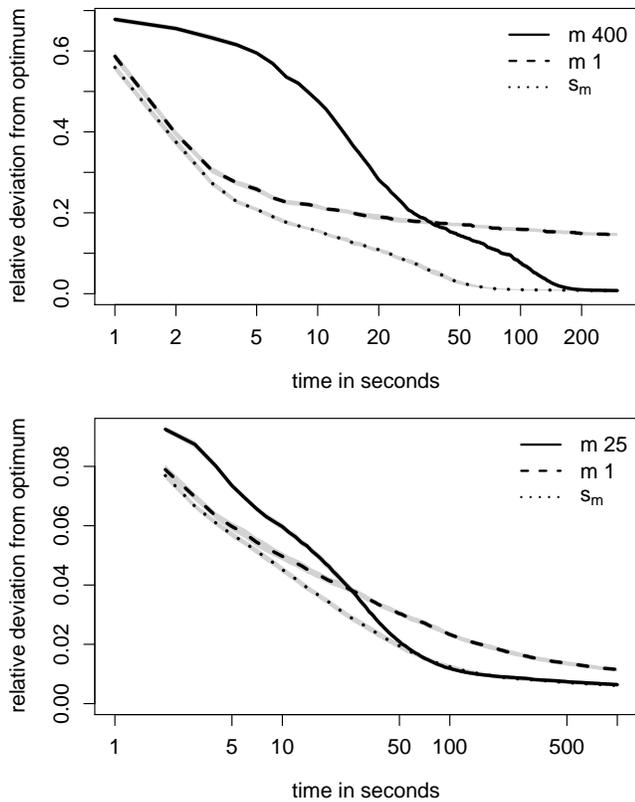
Fig. 1. Comparison of fixed and pre-scheduled variation of parameter  $m$  for MMAS (top) and MMAS+ls (bottom). The pre-scheduled parameter variation ( $s_m$ ) starts at  $m = 1$ , adding one ant every ten iterations.
