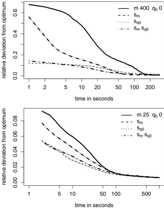
Fig. 3. Pre-scheduled variation of both parameters  $m$  and  $q_0$  in MMAS (top) and MMAS+ls (bottom). The variation schemes are the same used in Figs. 1 and 2.
