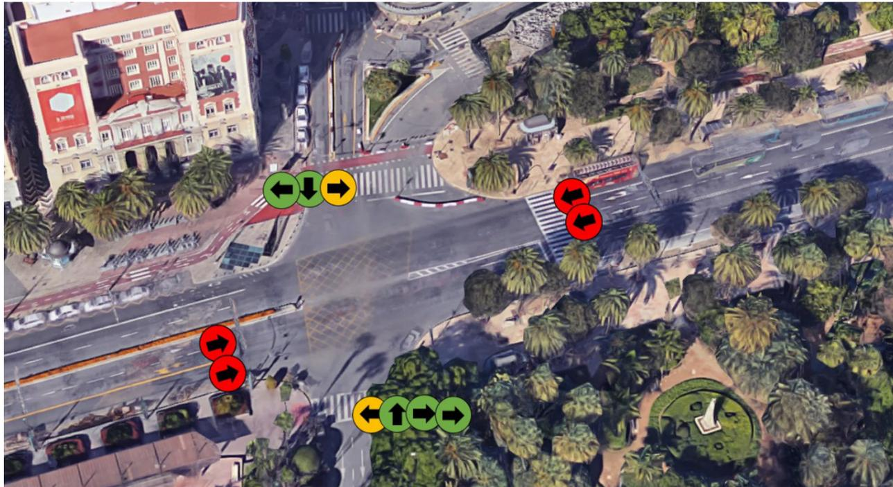
Figure 1: Example of one phase of traffic lights within an intersection. Clock-wise from left-most: “rr ggy rr yggg”.
