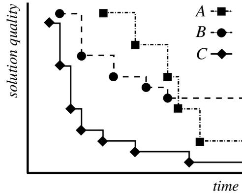
Figure 1: Performance profiles of three algorithms  $A$ ,  $B$ , and  $C$  (or three independent runs of the same stochastic algorithm).
