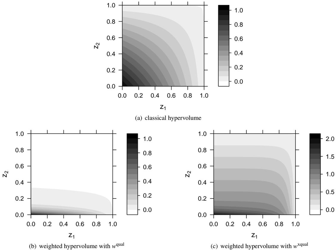
Figure 5: Value of the classical hypervolume (a) and the weighted hypervolume when using weight functions  $w^{\text{qual}}$  (b) and  $w^{\text{xqual}}$  (c) on the normalised objective space. The grey level at each point gives the (weighted) hypervolume of that individual point, which is computed as the integral of the weight function over the region dominated by the point and bounded above by the reference point (1, 1).
