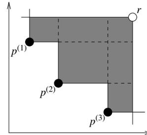
Fig. 1. The hypervolume indicator in the two-objective case
